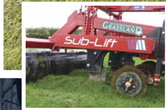
Serrated blades slice open the pan
